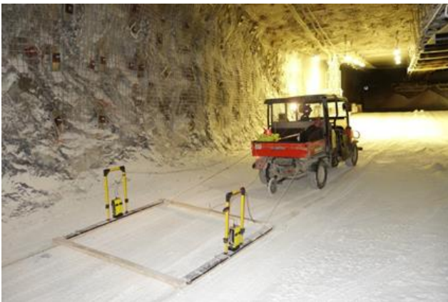
Fig. 4. The "sled" used to collection 50 MHz GPR.
